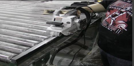
Then using a Porter Cable with a 100 grit sand belt sand the top and edge of the piece.
