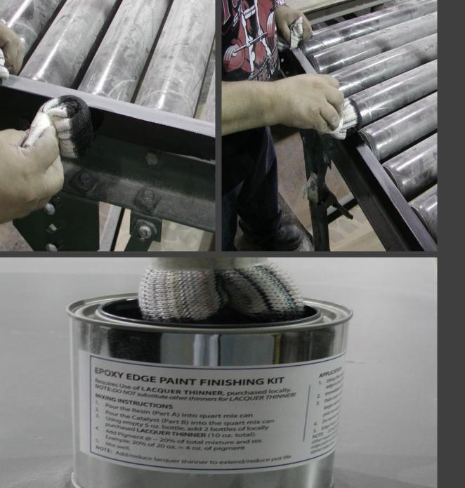
• Then using the epoxy edge paint proceed to paint the sanded edges. Be sure to follow the instructions on the quart can.
