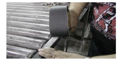
• After sanding with the porter cable use a sand belt and blend in the area that has been sanded.
