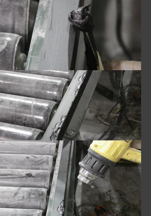
• Then using a heat gun start to heat up the smooth-on be sure to keep the heat gun at least 6 inches away from the patch. Placing the heat gun to close may cause the adhesive to gum up. If you don't have a heat gun let the smooth-on harden on its own this could take up to 6-8 hours depending on the temperature.
