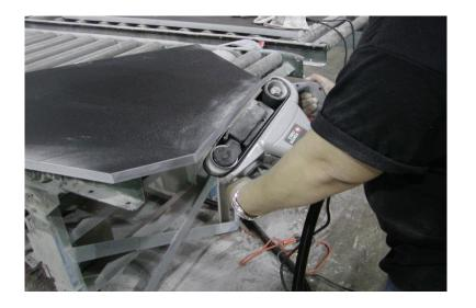
After sanding the edge tilt the sander and break the bottom edge usually 1/8" edge break. Than repeat the process on the top edge. Be sure not to apply to much pressure or the belt may dig into the material.
